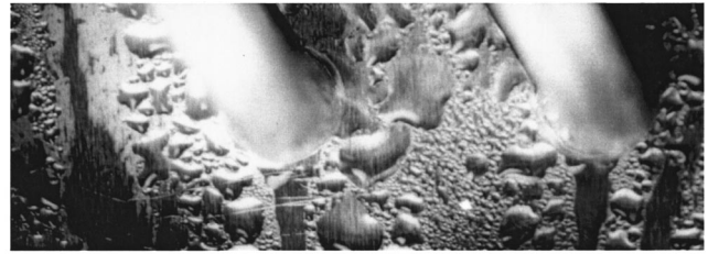
Fig. 10 This photograph shows a typical droplet distribution on the plain-fin heat exchanger after more than 100 hours exposure to condensing condition. This image was recorded under the same conditions and at the same location as that shown in Fig. 5.
